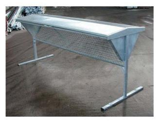
The freestanding hay rack is 8ft long and is constructed using 2" x 2" or 3" x 3" mesh infill with reinforced edges, 50mm x 25mm box frame and 16<sup>th</sup> plate endcaps and optional trough. The lid is hinged and held in the open position using a galvanised chain. All items fully galvanised after manufacture.
